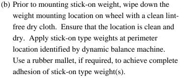
**NOTE:** Maximum stick-on type weight is **200 g** (7.0 oz.) inner and **200 g** (7.0 oz.) outer. If removal and replacement of stick-on type weight is necessary, then remove the weight using a nylon removal tool.
